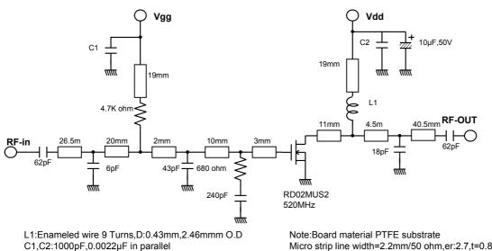
Micro strip line width=2.2mm/50 ohm,er:2.7,t=0.8mm
