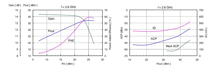
Bias conditions: VDD = 10 V, IDQ = 400mA, Frequency: 2.6 GHz Modulation Signal: 3GPP TEST MODEL 1 (W-CDMA) Reference plane: Connector Edge
