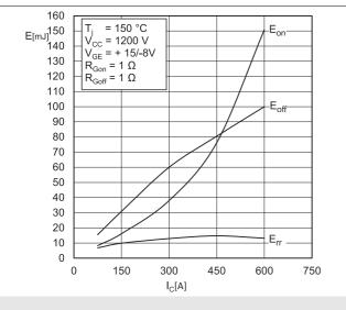
Fig. 3: Typ. IGBT1 & Diode2 turn-on /-off energy = f ( $I_C$ )
