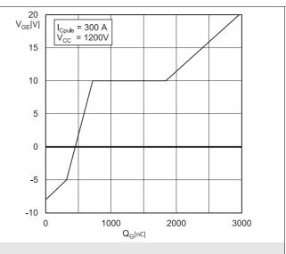
Fig. 6: Typ. IGBT1 gate charge characteristic
