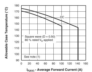
Fig. 5 - Maximum Allowable Case Temperature vs. Average Forward Current (Per Leg)
