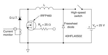
Fig. 8 - Unclamped Inductive Test Circuit
