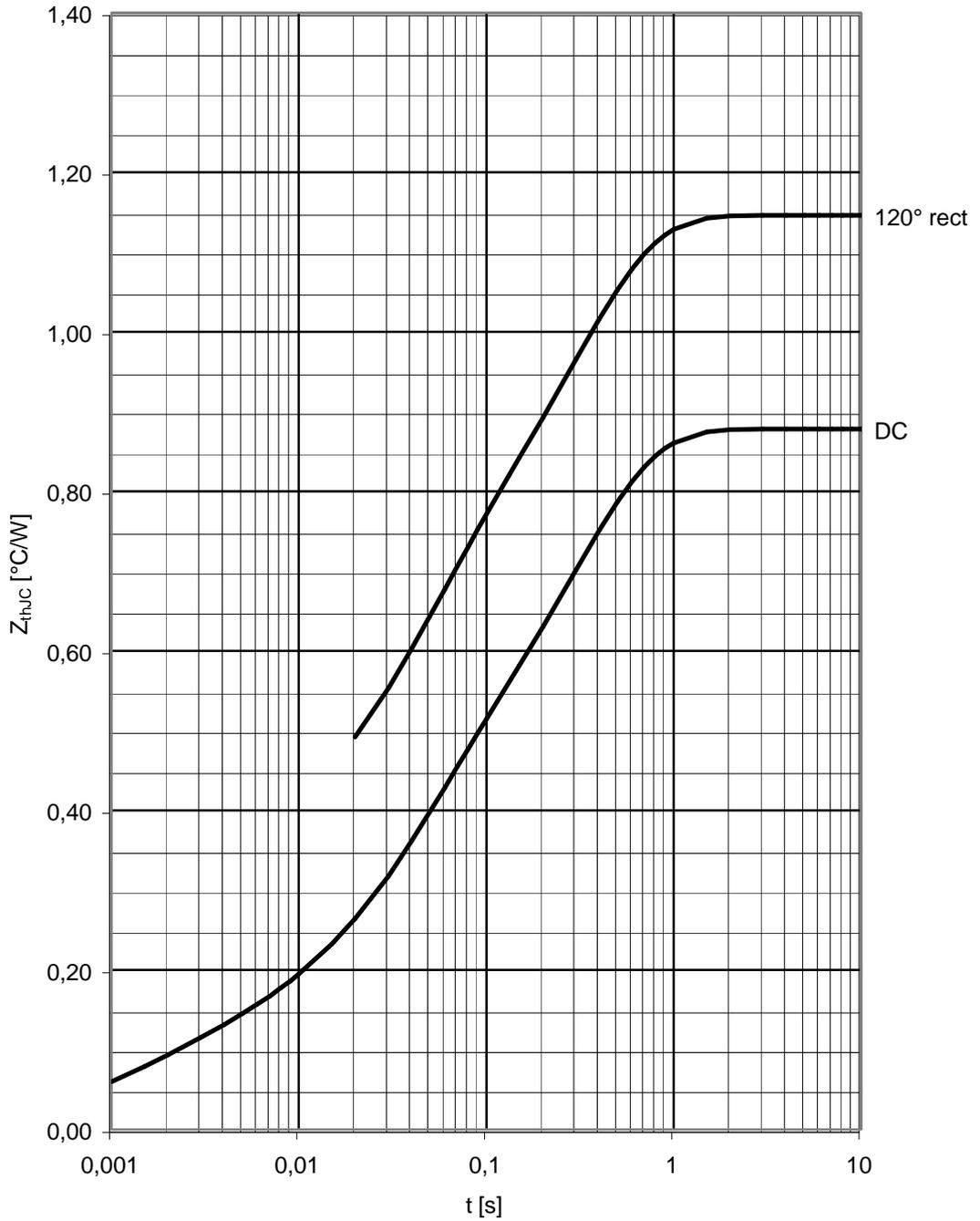
Transienter innerer Wärmewiderstand je Zweig / Transient thermal impedance per arm  $Z_{thJC} = f(t)$
