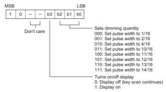
Note: power-on status: 1/16 pulse width is set and the display is turned off. Key scanning will be stopped during power-on status.
