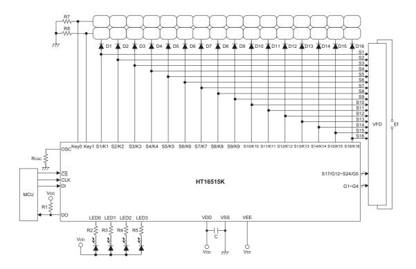
Note:  $R_{OSC}$ =82 $k\Omega$  for oscillator resistor
